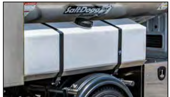
Integrated pre-wet system with LS15 (twin 80 gallon tanks) See pg. 56 for details
