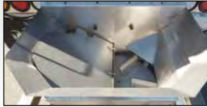
"Hex flow" chute and 24 inch spinner with adjustable baffles for optimal spread pattern
