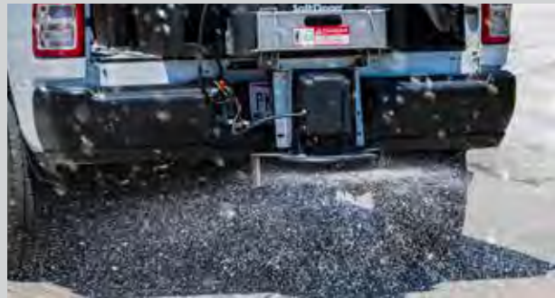
Two 12V direct drive gear motors (3/4 HP for auger or chain and 1/2 HP for spinner)
