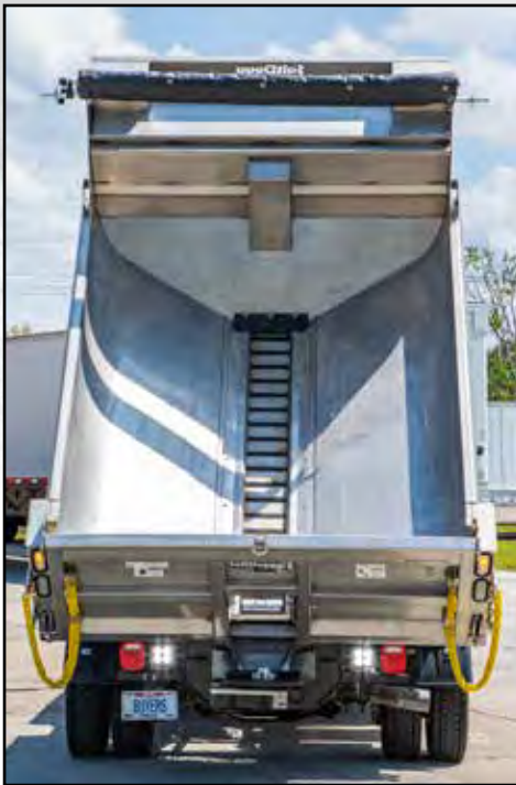
Cross member-free design makes the unit easy to clean with a low center of gravity that reduces strain on the vehicle
