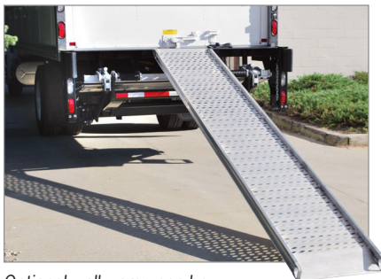
Optional walk ramp can be operated without moving the liftgate.
